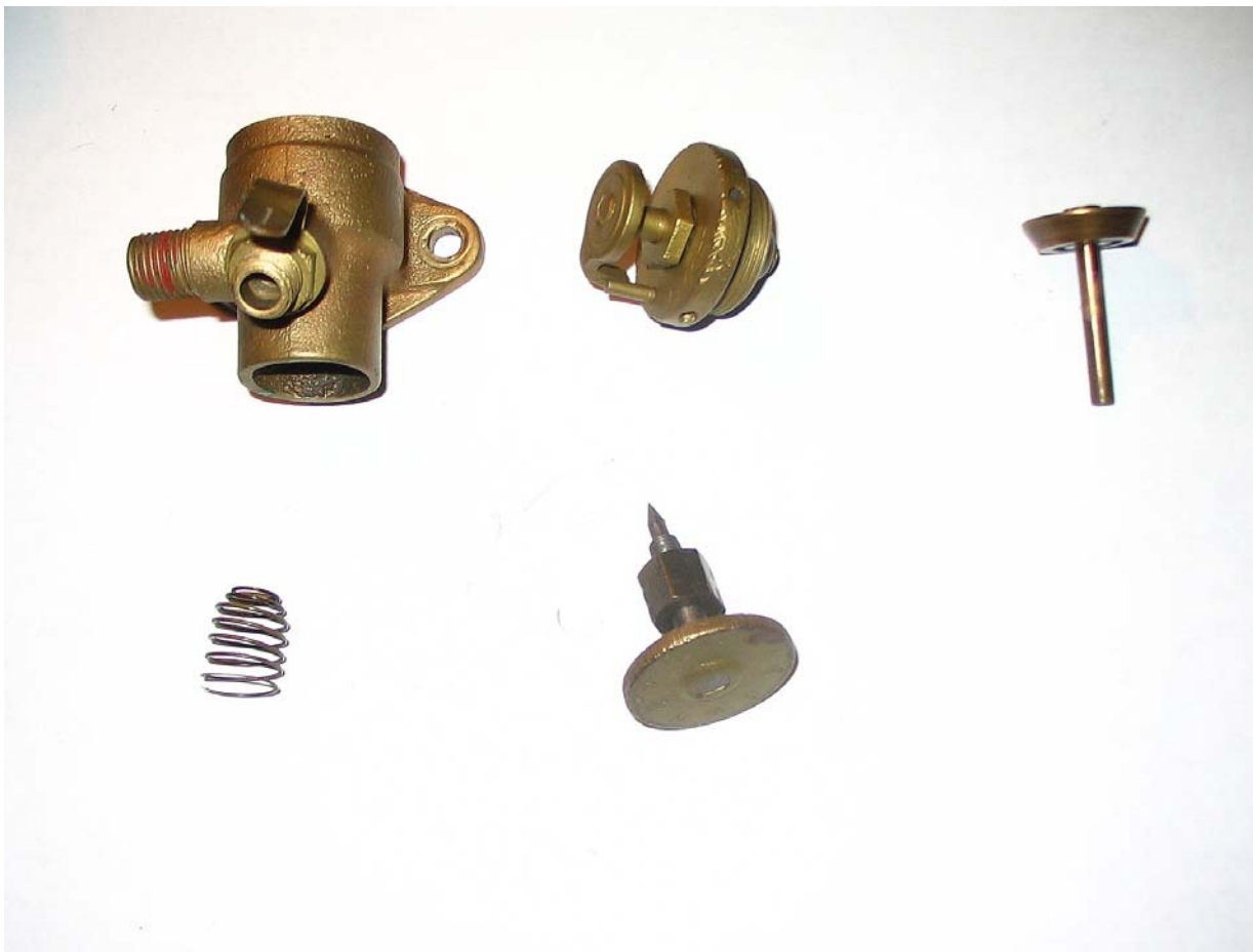
Figure 1 - Clockwise from top left - Mixer valve body; poppet valve chamber cap and travel adjustment knob; poppet valve; fuel needle valve assembly; and poppet valve spring. This mixer uses an internal valve spring.
