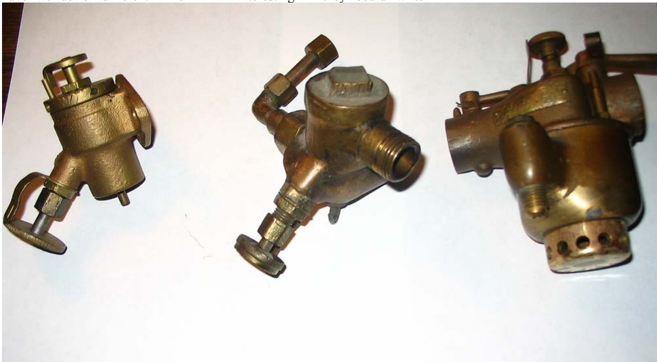
From left to right -Evinrude Rowboat Motor mixer valve with flange mount; Wisconsin rowboat motor mixer valve with a pipe-thread mount; four-ball Kingston float-feed carburetor.
